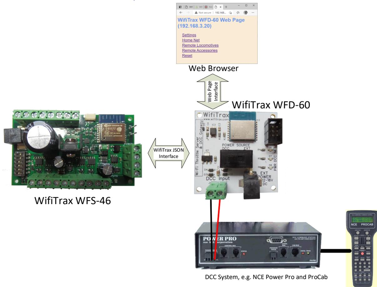
Figure 12 Controlling the WFS-47 using DCC such as an NCE Command Station/Booster
