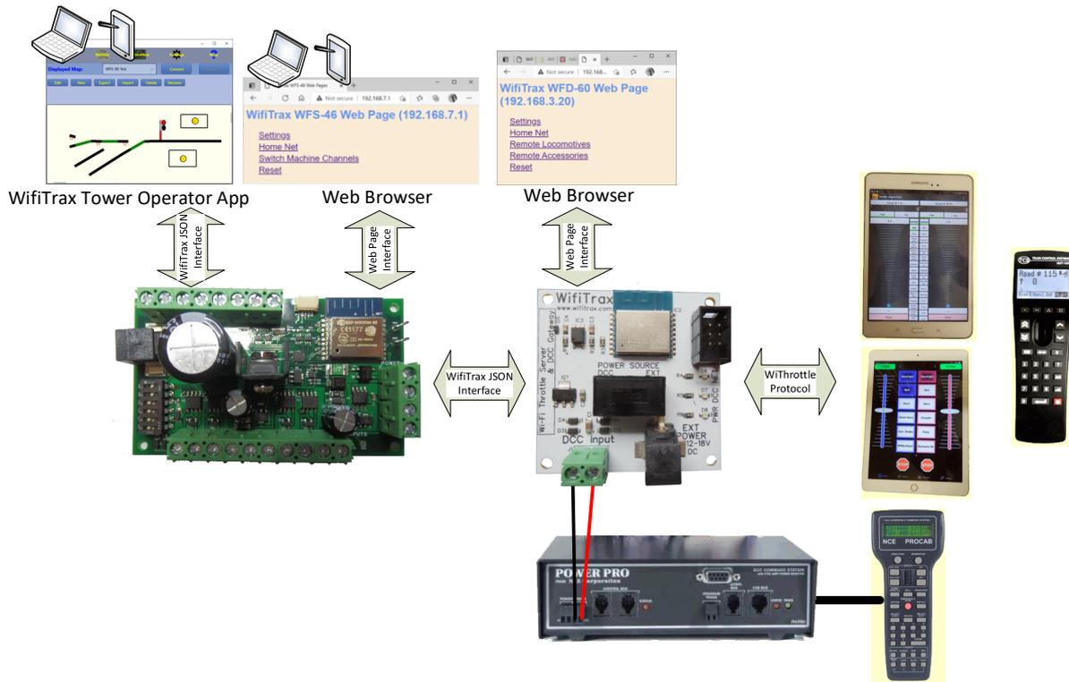
Figure 9 Options for control of switch machines using the WFS-47
