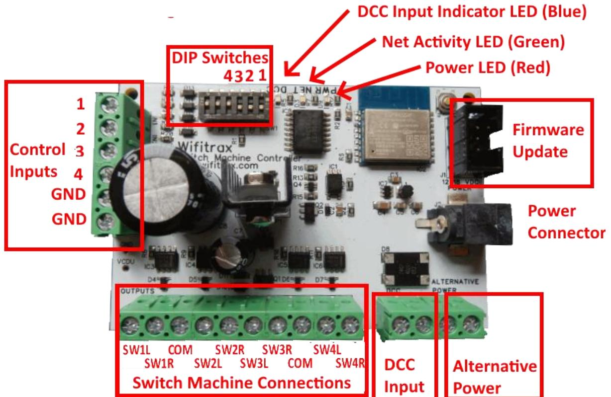
Figure 1 Connections and switches on the WFS-47
