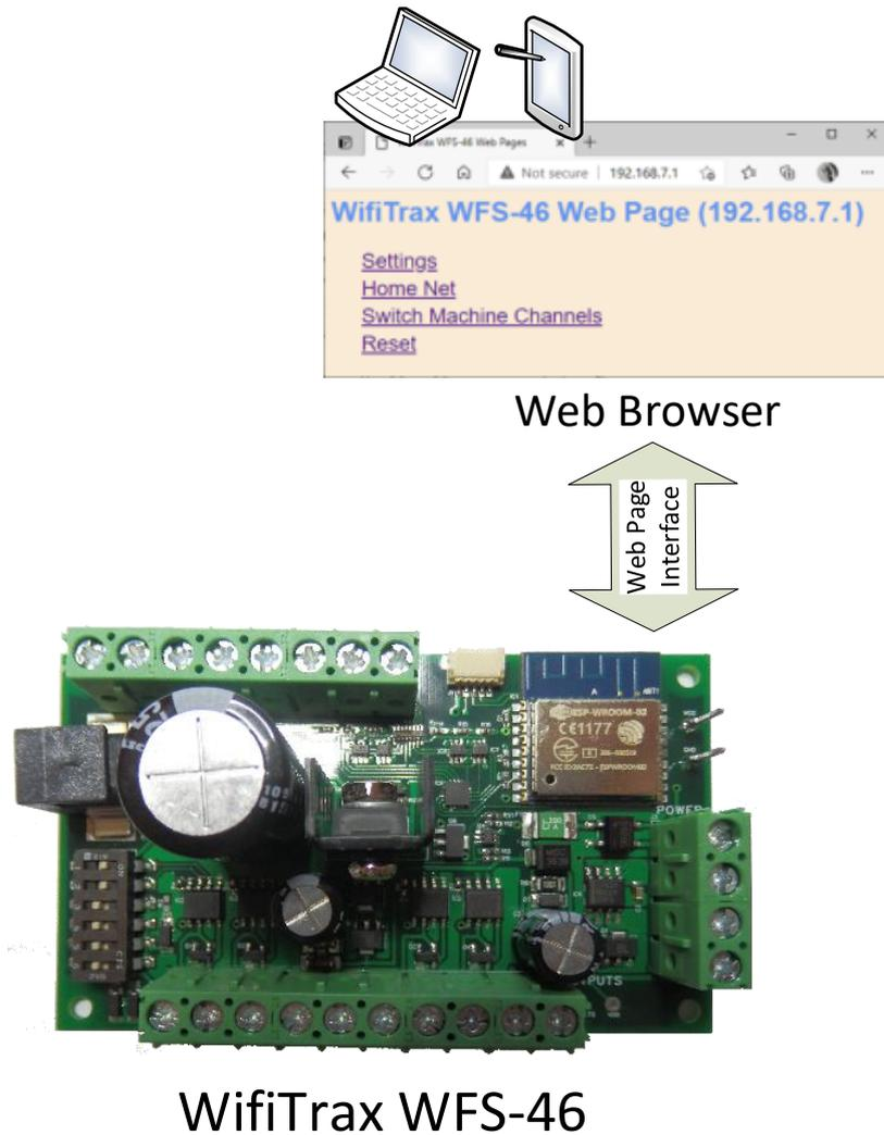
Figure 10 Control of WFS-47 using only its Web Pages
