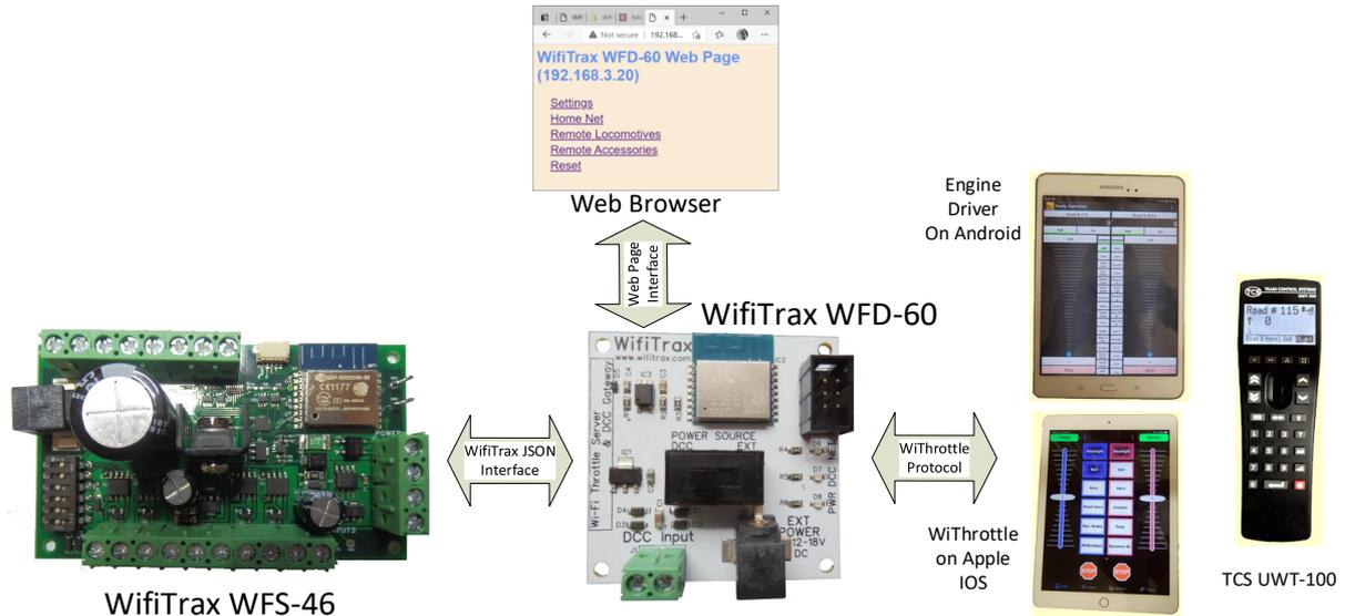
Figure 11 Controlling the WFS-47 via a WFD-60 and WiThrottle Protocol Devices
