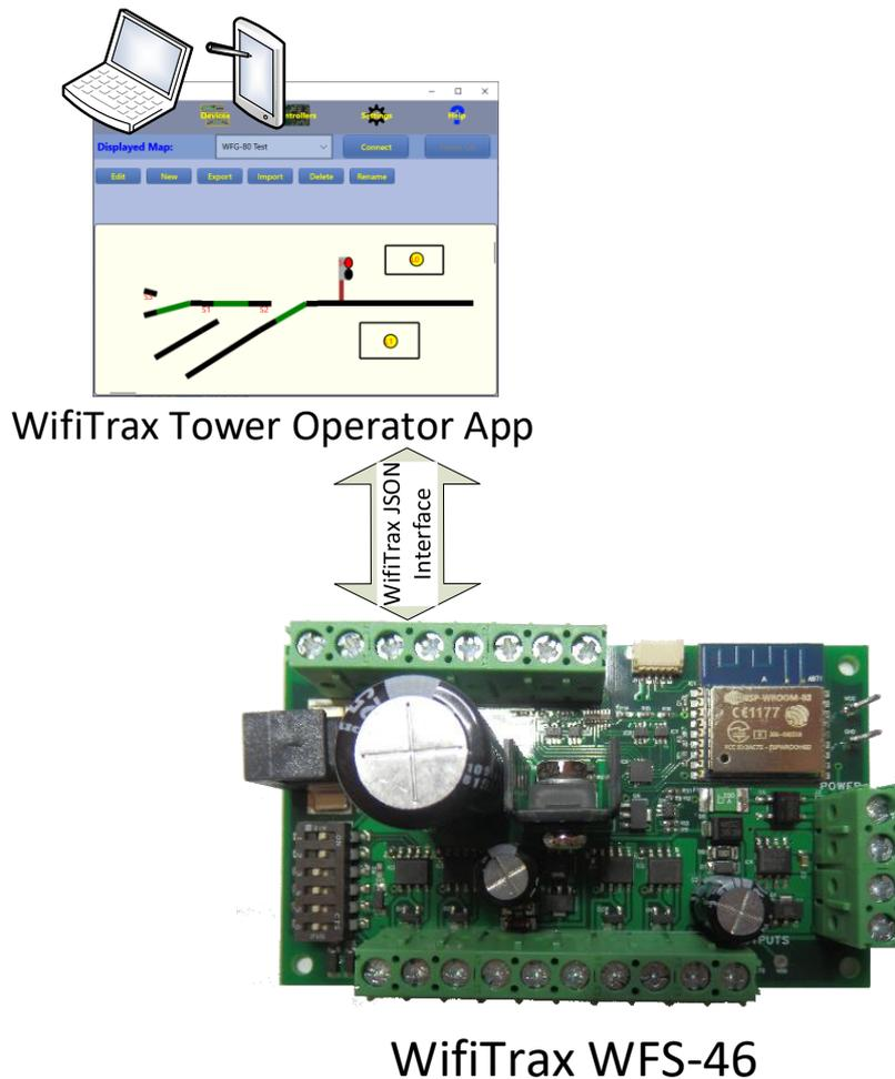
Figure 13 Using the WifiTrax Tower Operator App to control WFS-47 with turnouts and a Y switch
