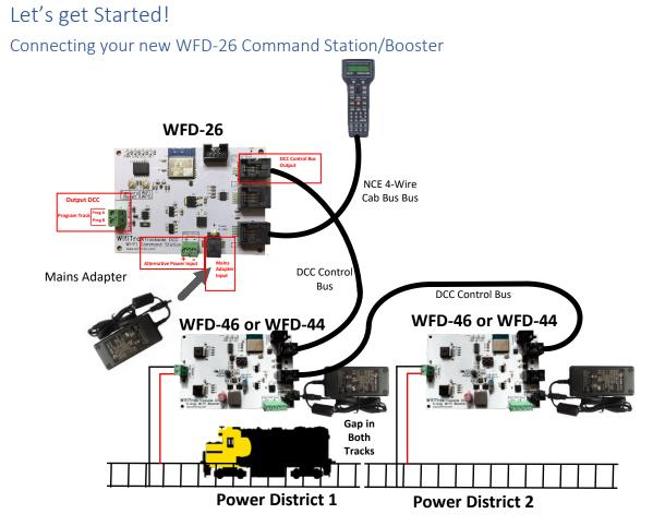
Figure 4 Connecting the WFD-27 Module to your Boosters, NCE Pro Cab, Track and Power
