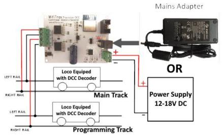
Figure 5 Connecting the WFD-27 Module to your Boosters, Track and Power
