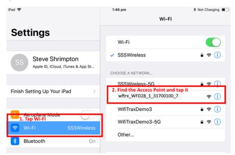
Figure 8 Connecting to the WFD-28 Wi-Fi Access Point
