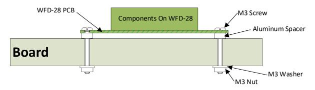
Figure 101 Mounting the WFD-2X on a board
