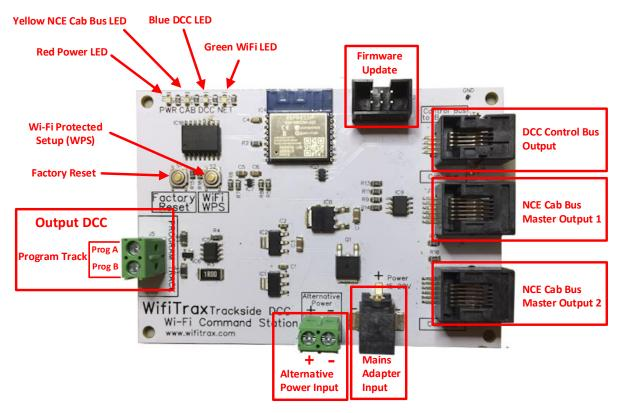
Figure 1 Connections on the WFD-26.
