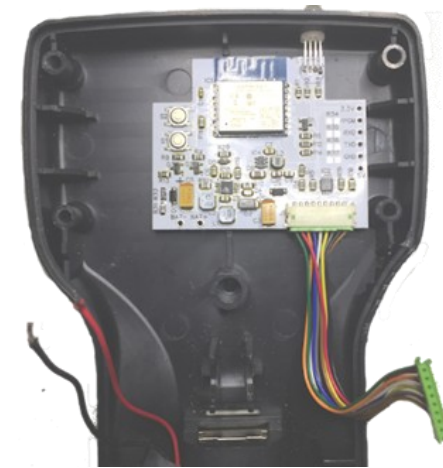
Figure 17 Fix the WNI-32 in position with its 9-way cable attached
