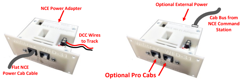
Figure 2. Left: PCP Mode connections to Power Cab. Right: UTP Mode connections to a Power Pro Command Station
