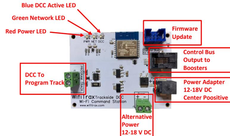
Figure 1. WFD-28 Connections
