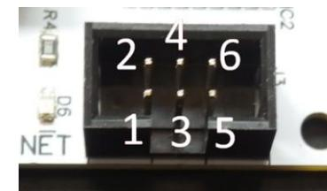
Figure 2. Header Connector on typical WifiTrax Module, pins numbered 1- 6.
